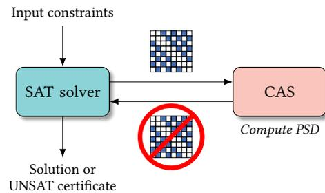
Fig. 9. A outline of the SAT+CAS method as applied to searching for Williamson matrices. The matrix provided to the CAS is blocked when it has a PSD value that is too large.
