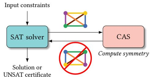
Fig. 5. An outline of the SAT+CAS method as applied to searching for projective planes. The SAT solver provides a partial projective plane to the CAS which computes the symmetries present. This example shows blocking the symmetry of rotating the partial plane by 180 degrees.
